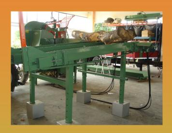
Ryetec Log Loaders are designed to link into your processor hydraulic system and run in tandem with your infeed conveyor. Log decks come as 1.2 metres or 1.4 metres wide and with the option of 3, 4 or 5 metres in length. Our Log Decks are designed to save time by loading a lot of timber in one go rather than loading single logs at a time.
