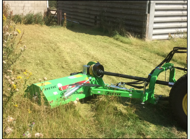
Heavy Hammer Flail on MUMH Lighter Delta Flail on MUML
