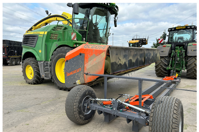
Hydraulically lowering trailer, with optional rear steer
