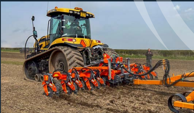
Restorer 6m ALD with hydraulic linkage working as a toolbar
