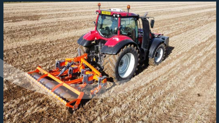
Restorer 3m ALD-E stand alone low disturbance sub soiler
