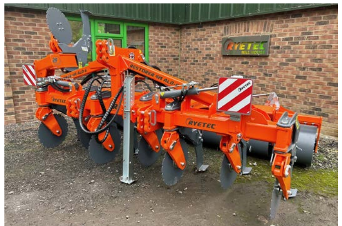
4m ALD-E with the ability to fold and work at 3m
