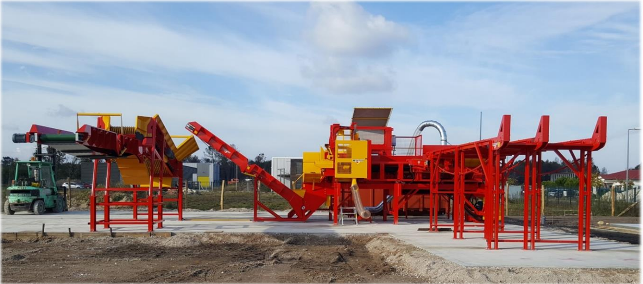
Xylog 600 with deck 6+2m; discharge conveyor 4+1m; feeding conveyor+wood screener and discharge conveyor
